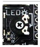
The LEDs on the RCD can be dimmed or brightened by adjusting a trimpot. Use a very small phillips screwdriver (#00 or #000) to adjust the trimpot. Be careful and gentle as you adjust the trimpot. It's safe to adjust the trimpot while the RCD is powered on, but be careful not to touch any components or solder junctions on the board.
