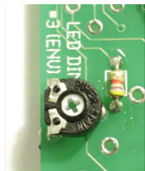
Above: 100k trimpot on far left edge Above: two 2N7000's on the top edge, left side
